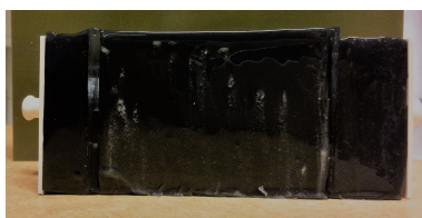
Figure 4.12: An image of the final phantom exhibiting the longitudinal movement.
