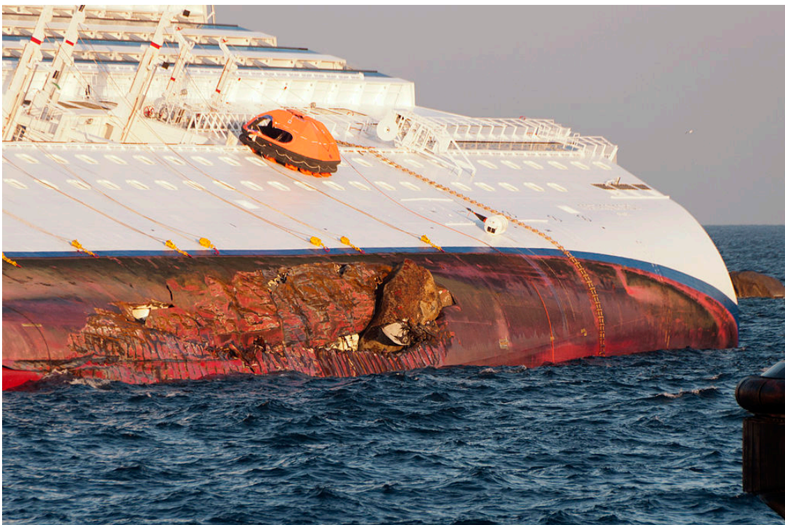
Figure 6 The impact with the reef tore a 53-meter long hole to the portside of the hull. A big rock was detached from the reef and got stuck in the hull of the vessel (image retrieved from Wikimedia Commons, photo: Roberto Vongher)
