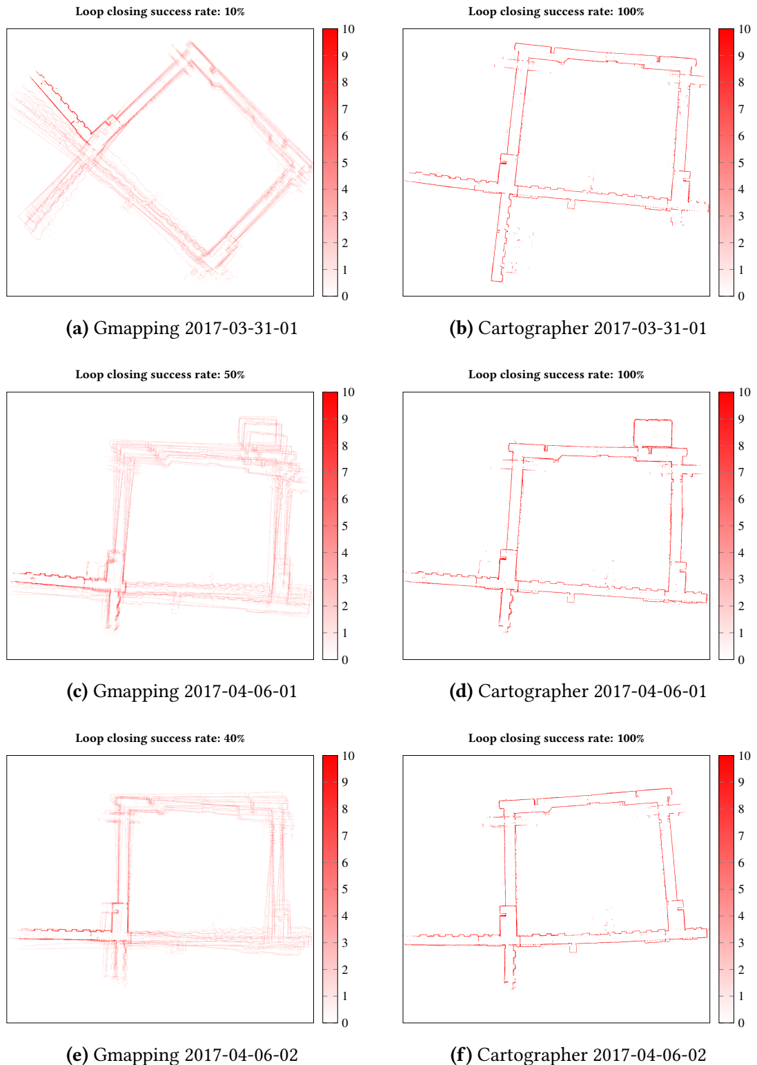
Figure 3.3: Visualisation of the different outputs from multiple runs of the same algorithm on the same data sets. Notice how Gmapping produces different maps every time while Cartographer does not. Notice also how Gmapping fails to close the loop and how Cartographer succeeds, but distorts the map in the process.
