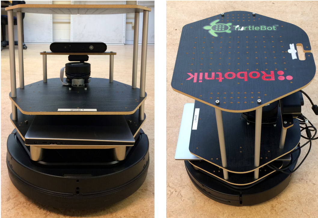
Figure 1.2: The Turtlebot used for the project. Note the base's similarities to commercial robot vacuum cleaners.
