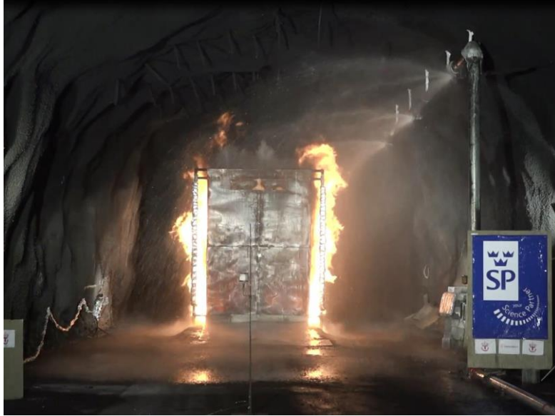
Figure 2 Test setup and FFFS after activation. With permission of SP [4]
