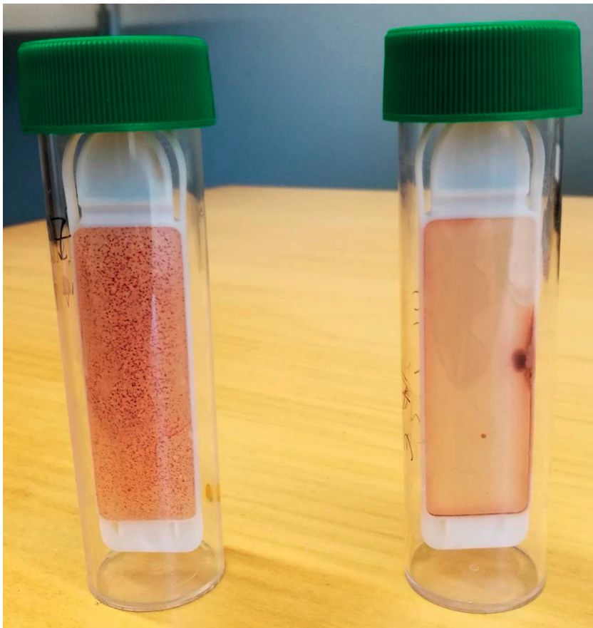
Figure 17. Two dip slide samples where the left one is the UF permeate from the 13th of March and the right one is the NF90 permeate from 9th of March
