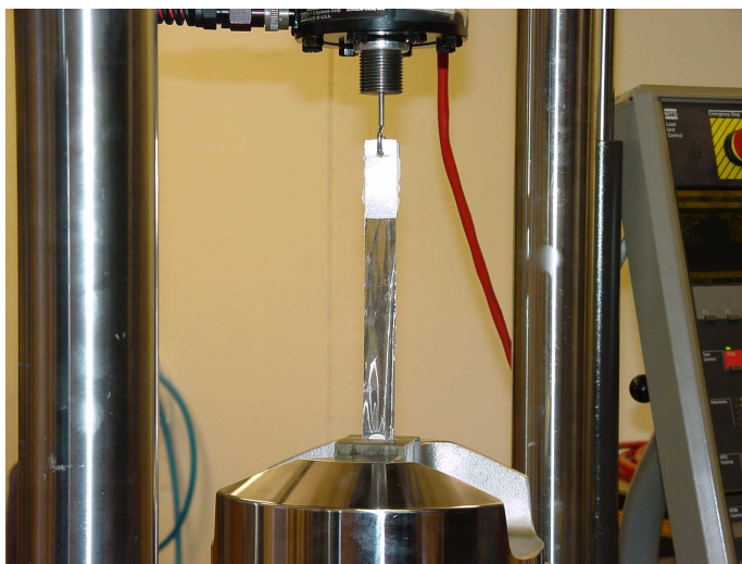
Figure 5.13: Creep test set-up of aluminium in a MTS.
