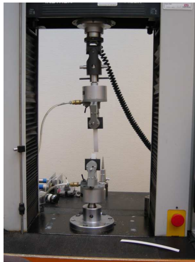
Figure 5.3: A uniaxial tensile test set-up in an Instron 4400R device.
