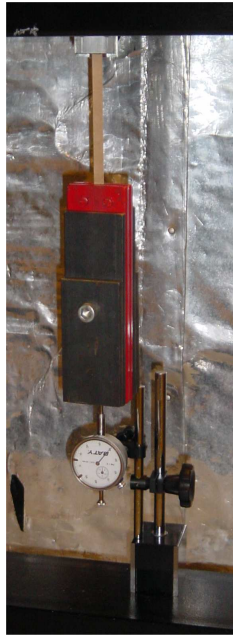
Figure 5.6: Creep test set-up of paper.
