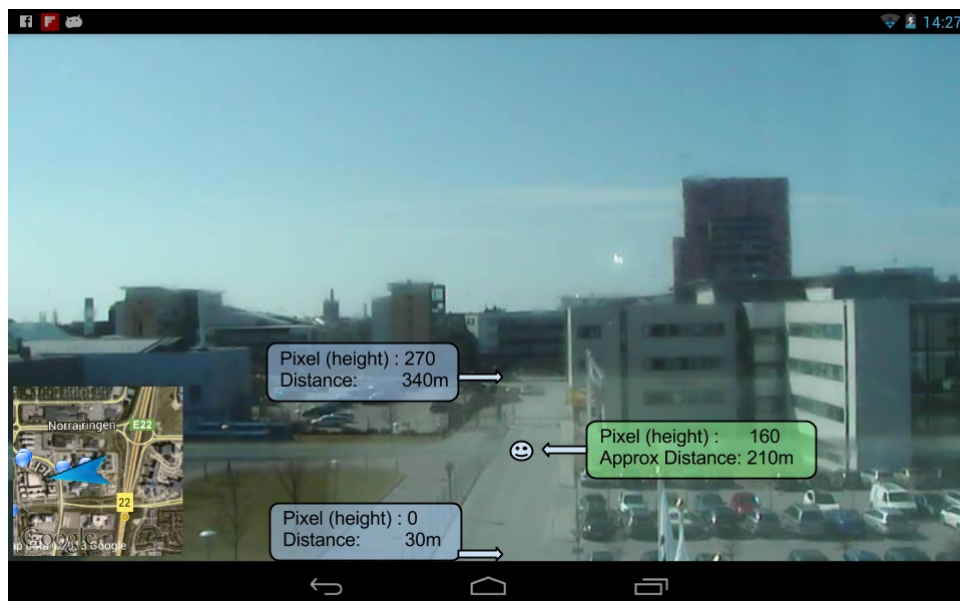
FIGURE 5.18: The process to go from screen-position to GPS-position.
