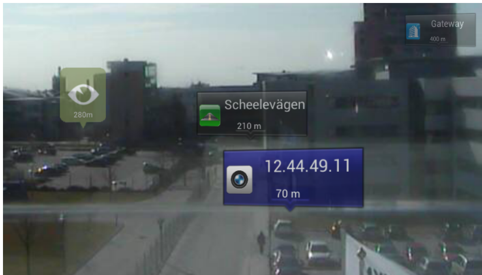
FIGURE 5.19: An object has been detected by another camera and displays its location in the current image.
