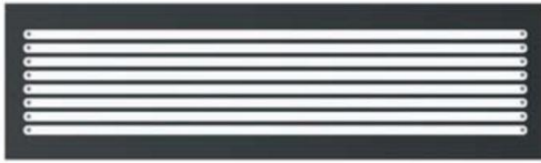
Figure 2. Illustration of a flow cell from Illumina. The flow cell in the picture is in approximately the original size. The flow cell has eight separate lanes.
