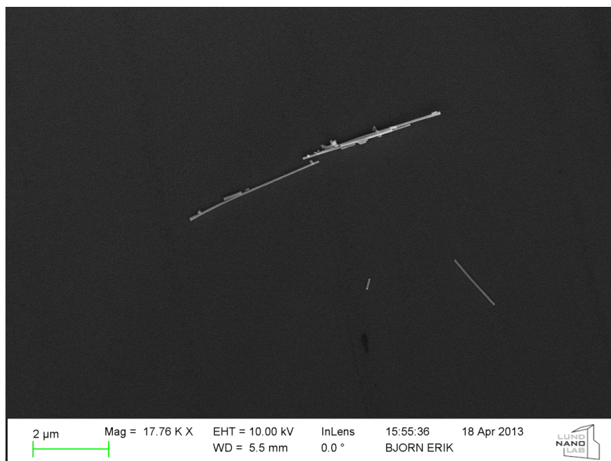
Figure 4.4 SEM image of the same area as in figure 4.3, the top wire is not a single wire but a cluster of wires and fragments of wires.
