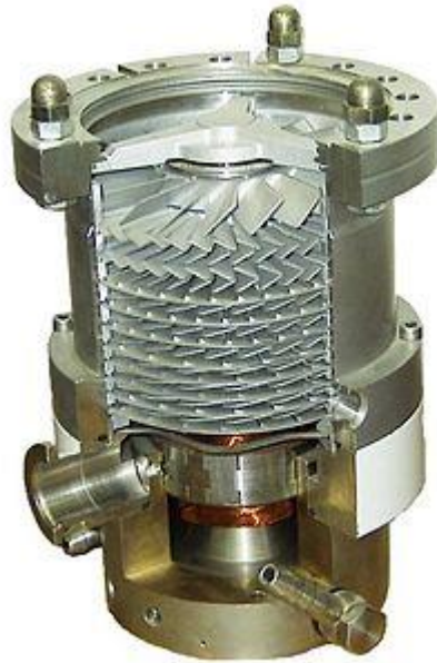
Figure 2.3 Interior of a turbomolecular pump. All the layers of rotating blades can be seen. Figure taken from http://en.wikipedia.org/wiki/Turbomolecular_pump , verified 2013-06-17. Author: liquidat
