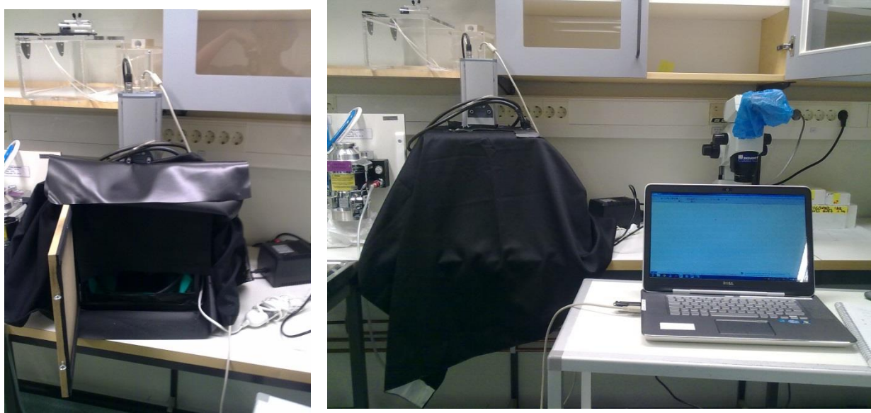
Figure 6 Left image: the CLI-box open with dark drapes pulled back. The object meant for imaging is placed at the bottom of the box directly underneath the CCD on the top of the box facing the bottom. A white light image of the object is taken this way and is later used to overlap the CLI images for an anatomical reference. Right image: The CLI-box closed and with the drapes pulled down to shut out ambient light. The CCD is connected to a laptop containing the software controlling its settings. When imaging, the overhead lights in the laboratory are switched off.
