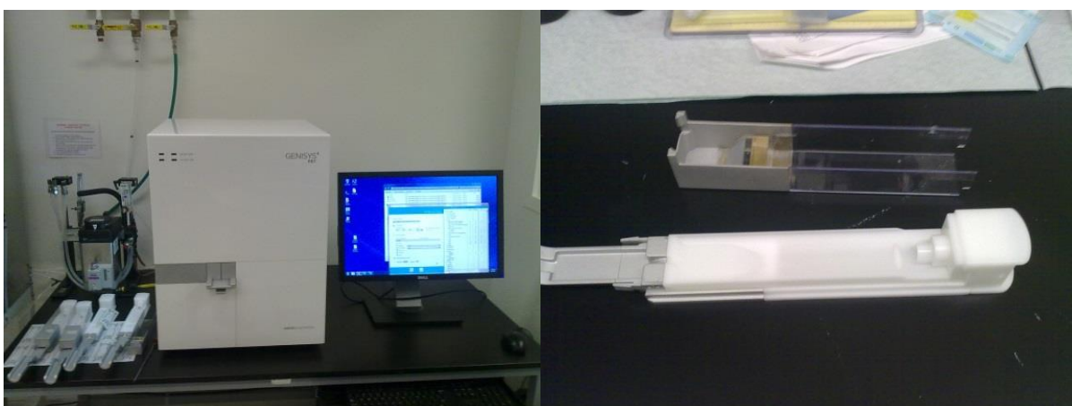
Figure 10 Left image: The Genisys4 PET-system (Sofie BioSciences) at the Ahmanson Translational Imaging Division at UCLA. Right image: the PET-systems mouse cradle in which the phantoms were mounted during the scan.
