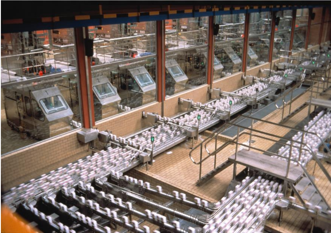
Figure 1 Production line using 11 TBA8 filling machines at Pascual, Spain
