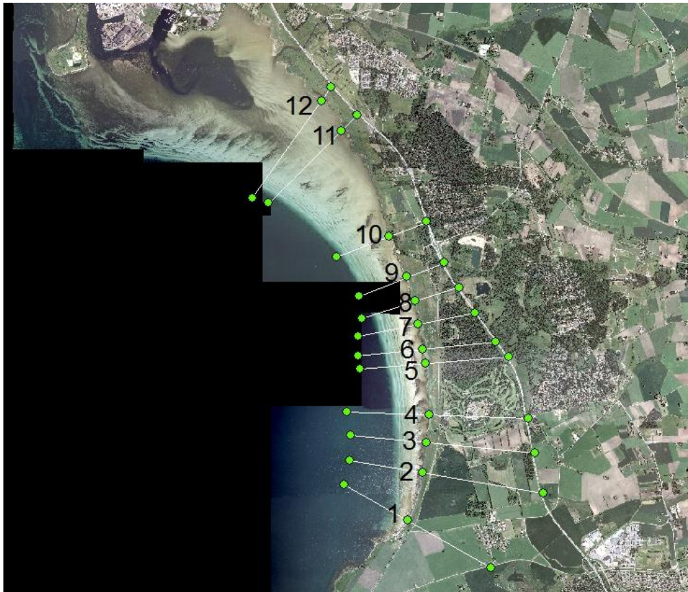
Figure 8. Modified orthophoto © Lantmäteriet, i2012/901. The profiles extracted from the Bathymetry and Topography Modelare marked, stretching from a depth of 6 m up to the highway (except for profile 1 that stretches up to another road). The dot in the middle of each profile marks the estimated location of the coastline.
