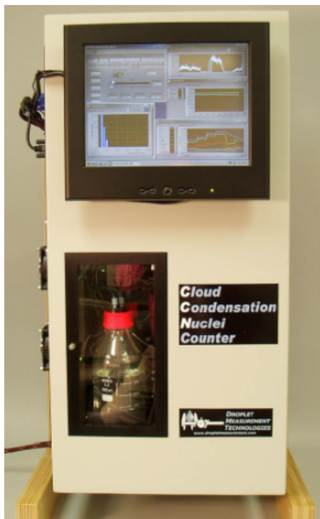
Figure 3: The Continuous-Flow Streamwise Thermal-Gradient Cloud Condensation Nuclei Counter from Droplet Measurement Technologies (CCNC DMT-100) [5].
