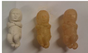
Figure 4.1: The model (to the left), the first molding (in the middle) and the second molding (to the right).
