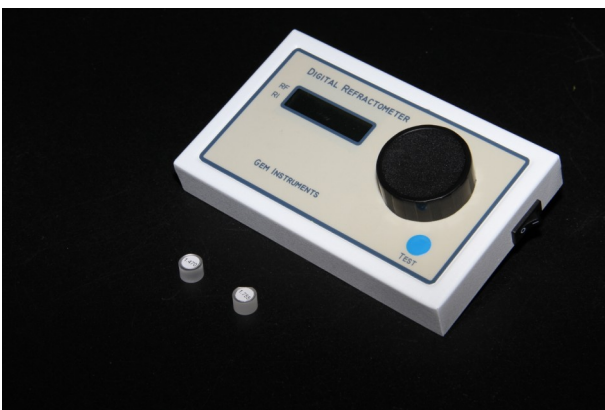
Fig. 2. The first generation infrared refractometer. Photograph: Ivan Suez.
