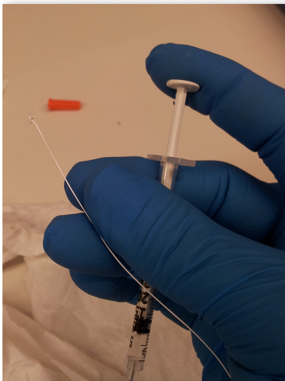
Figure 4a. The hollow fibre membrane was cut into 20 cm long pieces and filled fresh acceptor buffer. The ends were sealed by melting...
