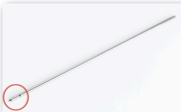
Figure 7. The Waters 2695 Separations module needle is constructed so that it picks up sample on the side, some 5 mm up from the needlepoint, rather than at the point itself, from [46].
