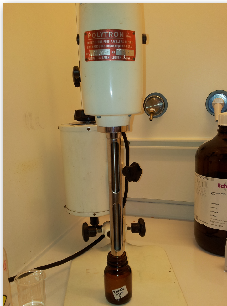
Figure 3. The fish/water mixture was homogenised for 10 minutes using a Polytron mixer.
