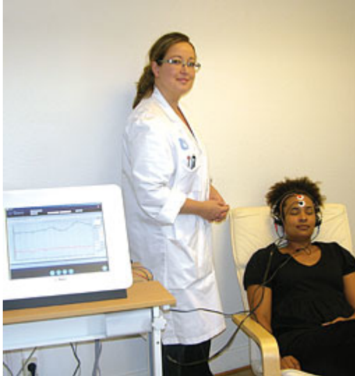
Figure 1.1: The figure shows the SensoDetect measurement set-up. Five electrodes are placed on the subjects scalp. Two behind the ears and three in the forehead. The subject then puts on a set of headphones, which play a click sound. The electrodes then measure the EP. The measurement session is conducted while the subject is simply sitting down in a chair in a dark, quiet room. Printed with permission from SensoDetect AB.
