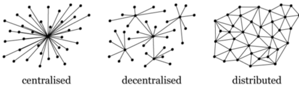
Figure 3-3. Centralized, Decentralized and Distributed systems
