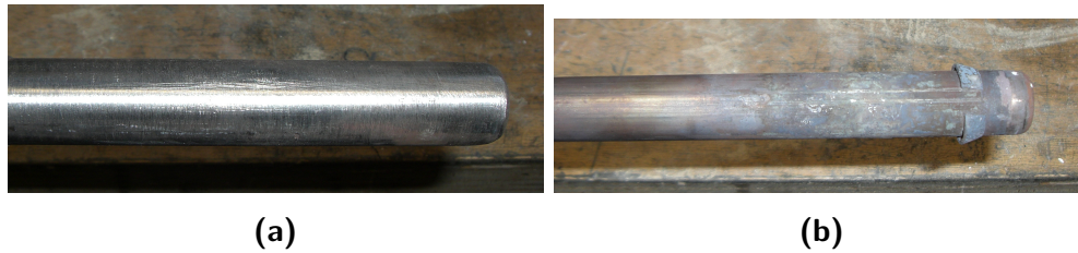
Figure A.14: Probe tip in different stages of the experiment: (a) Polished probe tip before experiment, (b) Probe tip after 30 minutes at 1400 °C and NaCl
