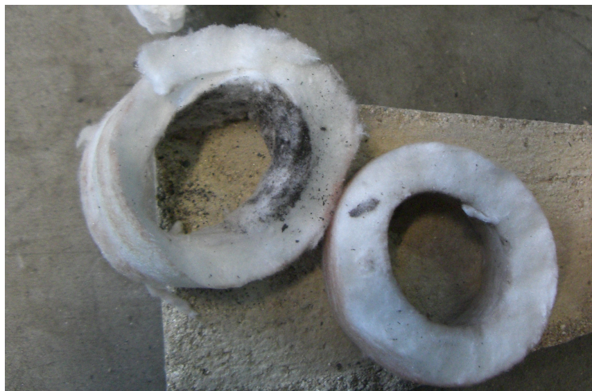
Figure A.16: Samples of the getter material after experiment at 1400 °C and 30 minutes exposure to NaCl
