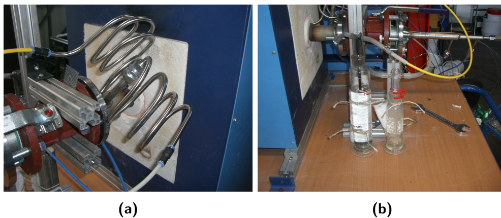
Figure 4.11: Photos of the (a) cooling tubes directly after the tube furnace and (b) impingers to protect the MFCs from alkali vapor
