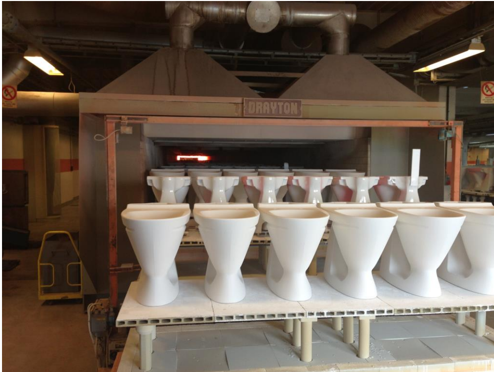
Figure 17 - Tunnel kiln 19, with bowls on a kiln car in front
