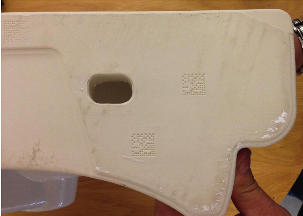
Figure 36 - Washbasin marked with Data Matrix on green ware, dried, glazed, and fired
