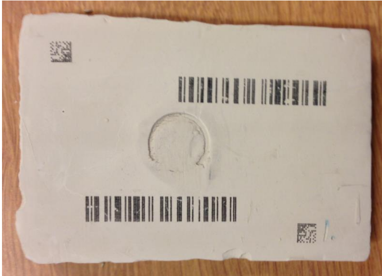
Figure 44 - 1D and 2D codes applied by CIJ ink jet on the underside of a sample
