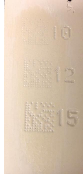
Figure 35 - Data Matrix marked on green ware, dried, glazed with a thin layer and wiped with sponge over the marks, then fired
