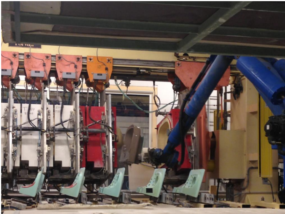
Figure 14 - An industrial robot demolds the piece in the casting cell, with green demolding plates in front
