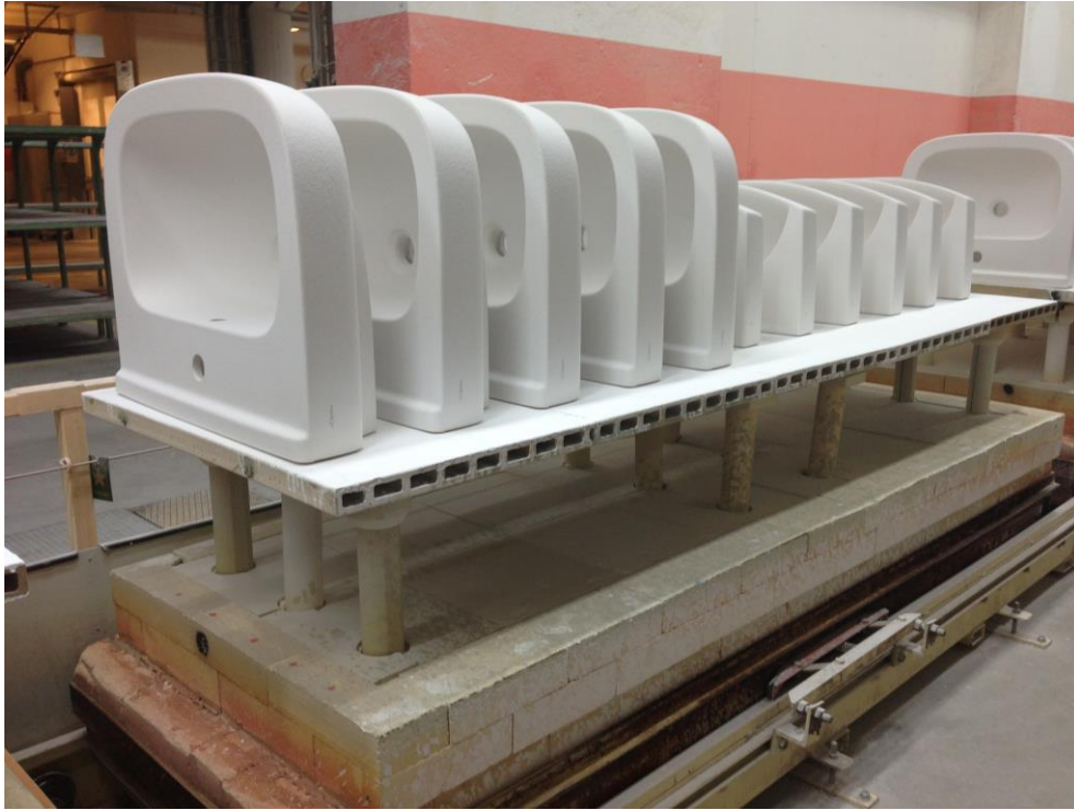
Figure 54 - Kiln car on a rail, leading it to a tunnel kiln
