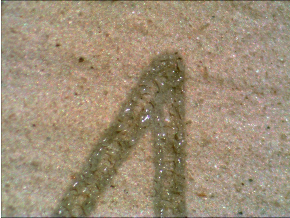
Figure 39 - Microscope snapshot of laser marking on dried ware
