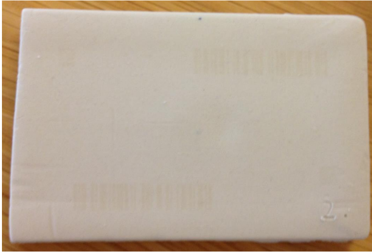
Figure 45 - 1D and 2D codes applied by CIJ ink jet on green ware
