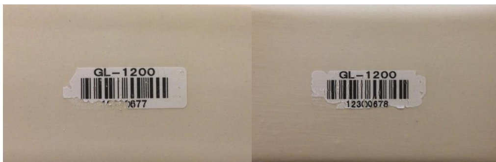
Figure 27 - The label was affixed to green ware, dried, and then fired.
