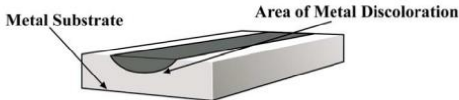
Figure 52 - Marking applied to surface using the laser coloration process (National Aeronautics and Space Administration, 2008a).
