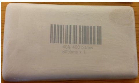
Figure 40 - Sample 1 - Dried VC marked with laser
