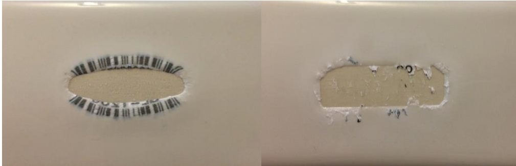
Figure 29 - The label was affixed to dried ware, glazed, and then fired.
