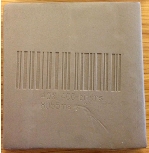
Figure 37 - Sample 5 - Bar code marked with laser on green ware
