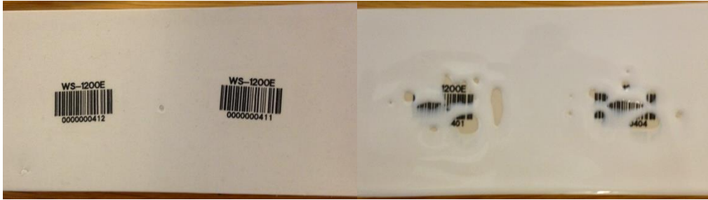
Figure 22 - Label applied to green ware, dried and then fired
