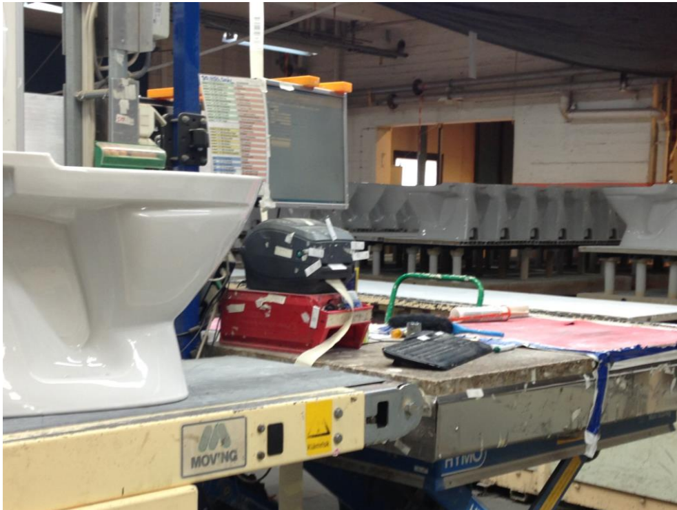
Figure 18 - Inspection station for VC-pieces
