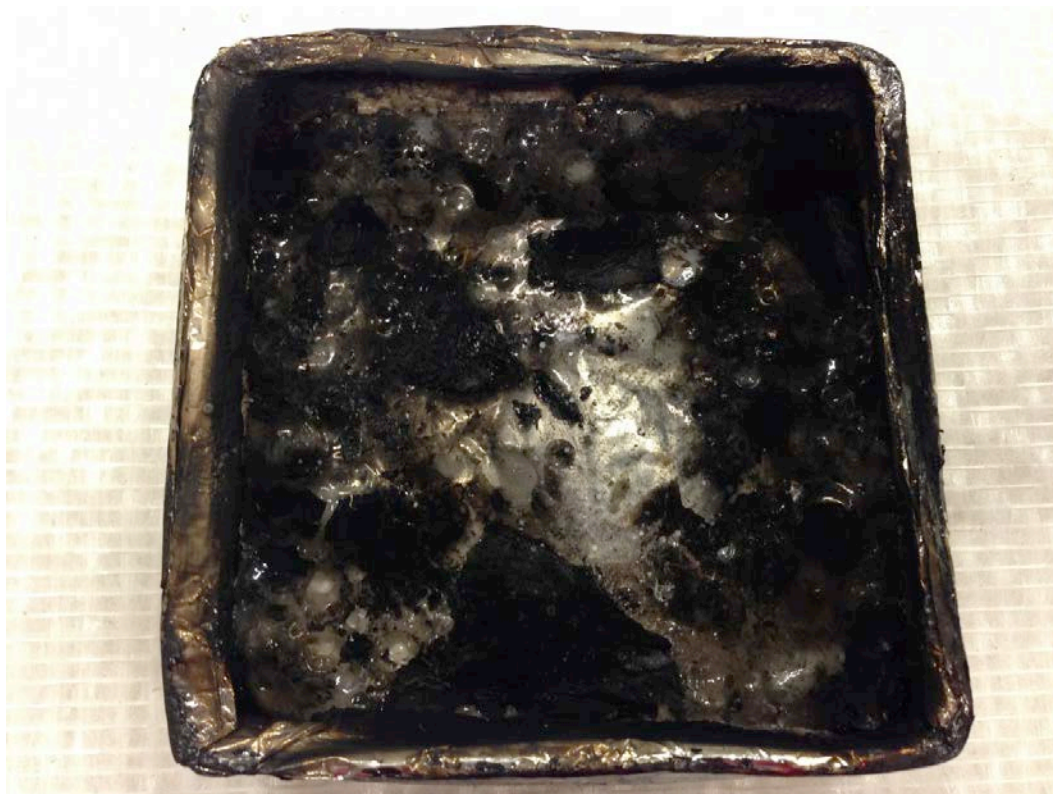
Figure 9 Colourless glass-like residue after combusting Borotron UH050.
