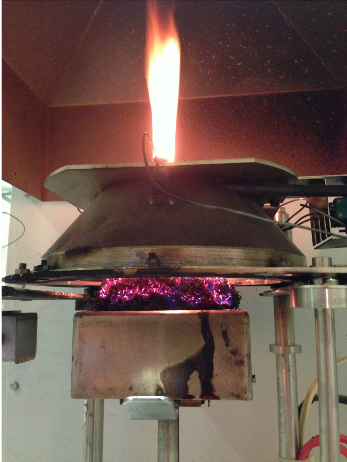
Figure 19 TIVAR Burnguard burning with a well-defined flame.
