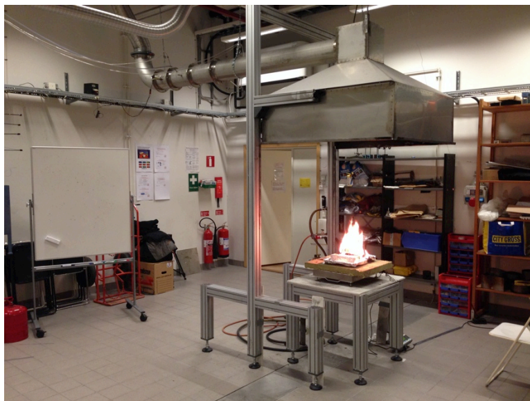
Figure 7 Burning material under the exhaust hood.
