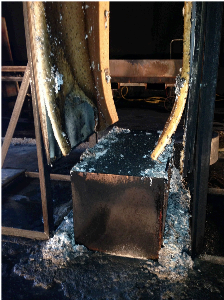
Figure 17 The melted material is piled up beneath the material plates.
