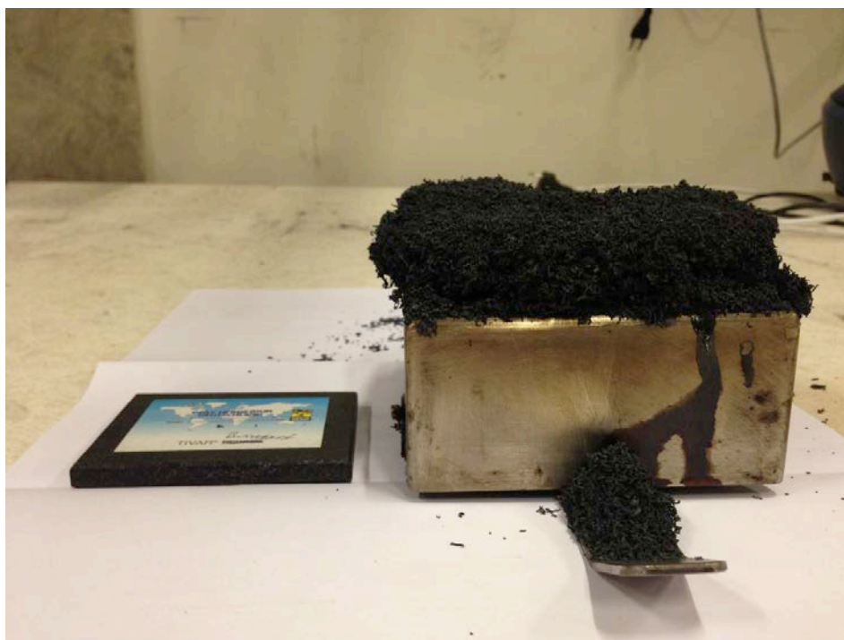
Figure 18 Comparison between the original size and the residues after combustion.
