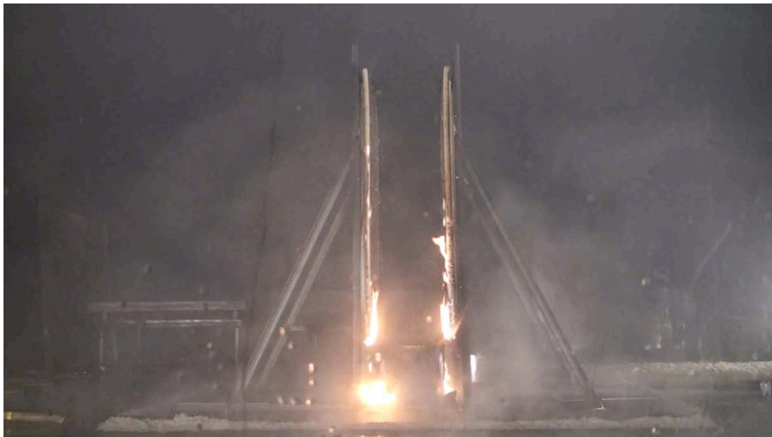
Figure 15 Small flames left after extinguish attempt.
