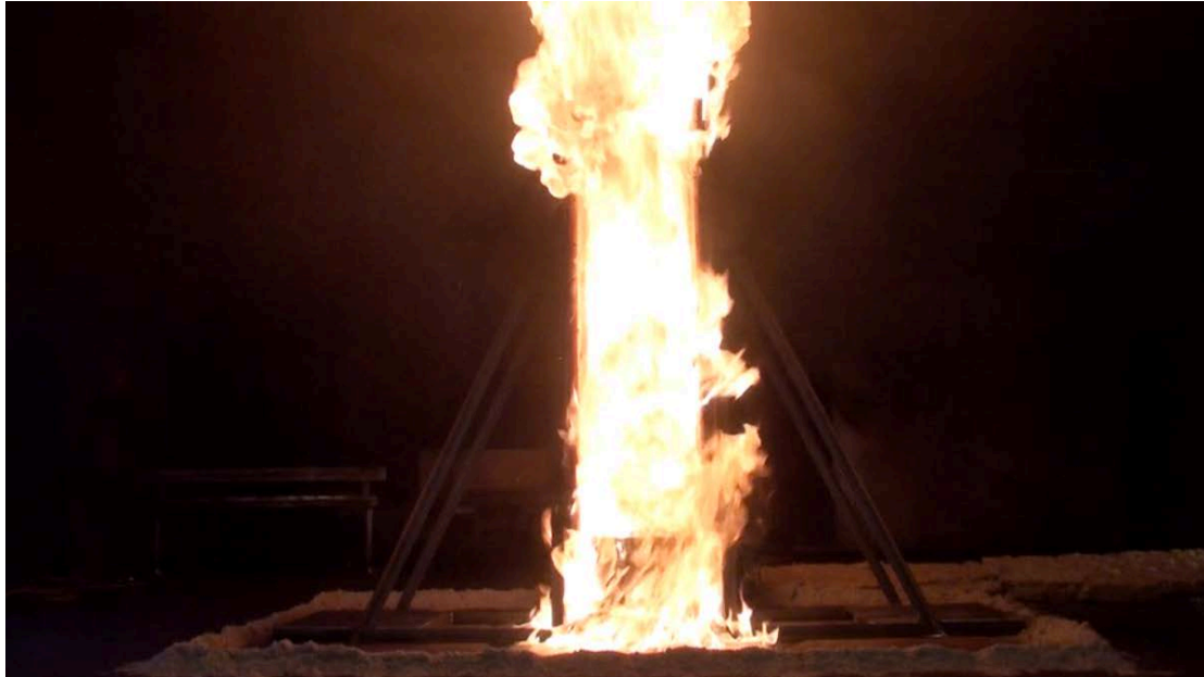
Figure 14 The whole area of the material plates is burning together with the melted material on the floor.
