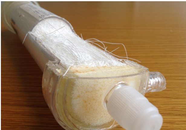
Figure 6.7 Cross-section of a dialyzer, showing the fibres through which the blood flows
