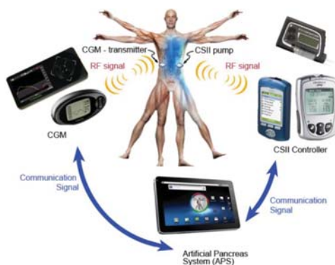
Figure 4. Overview of the UCSB/Sansum Artificial Pancreas System.
