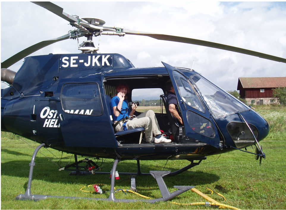
Figure 2.2.1. Preparing for taking aerial photographs from Eurocopter AS 350 B3 by flying with open back door and secured with harness. Pilot Michael Elmeskog. (Photograph by Tanja Zaubek)
