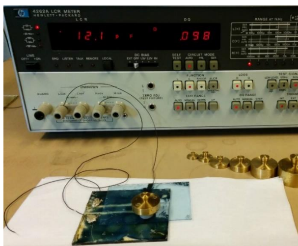
Figure 26. Calibration of the sensor, by placing known weights and reading out the capacitance on the LCR-meter.
