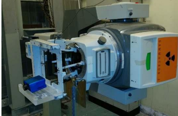
Figure 29. The Gammatron 3, used for radiation tests.
