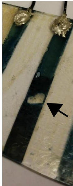
Figure 41. The middle PEDT pattern is not uniform, the arrow shows a part of the layer which consists of no PEDT at all.
