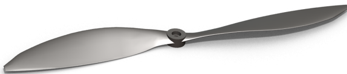
Figure 2.14: Rendered picture of an APC 10x4.7 Slowflyer propeller, modeled in Solidworks [27].
