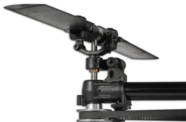
Figure 5.8: Implementation of a variable pitch propeller for the Stingray 500 quadrotor [25].
