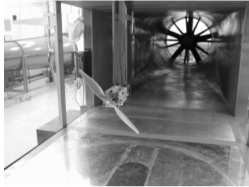
Figure 2.15: Experimental setup for the wind tunnel test conducted by [5].
