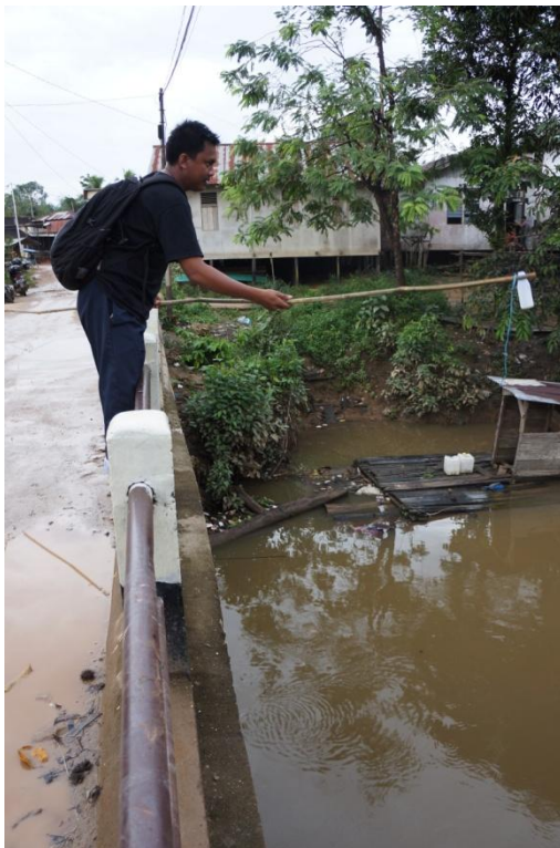
Figure 4.4.1. - Sediment sample taken at station 3. Test tube tied to a bamboo stick an lowered into the river.
