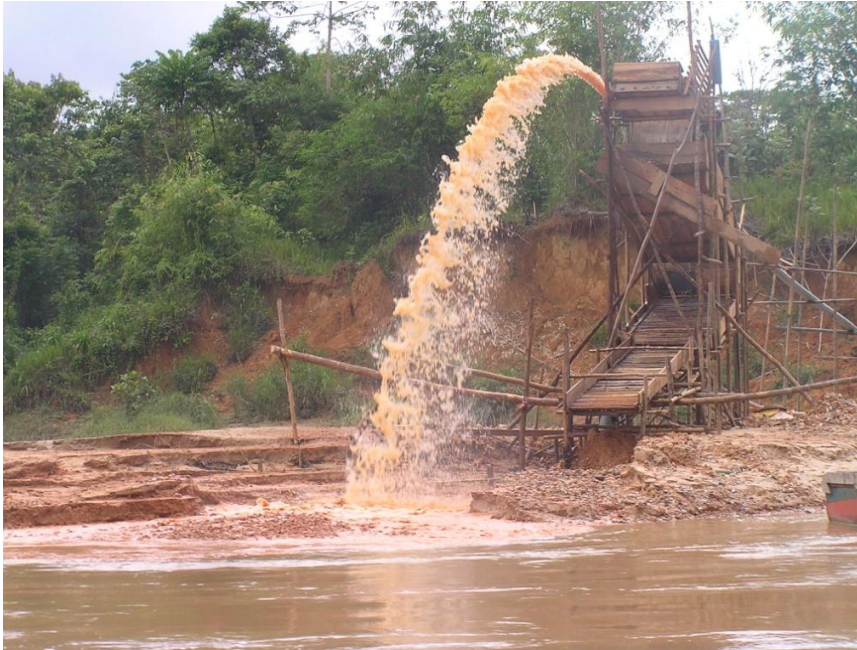
Figure 2.1.1. – Picture illustrating the process of mining. Used waste water is washed out into a nearby river resulting in large amounts of sediment transport. (Picture taken by lecturer at Lingkungan faculty, Tanjungpura University.)
