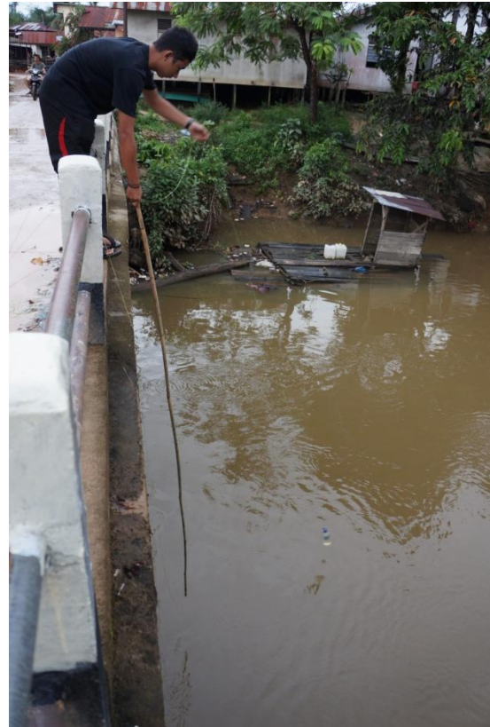
Figure 4.3.3.2. - Float tied to a long bamboo stick, used as velocity measurement at station 3.
