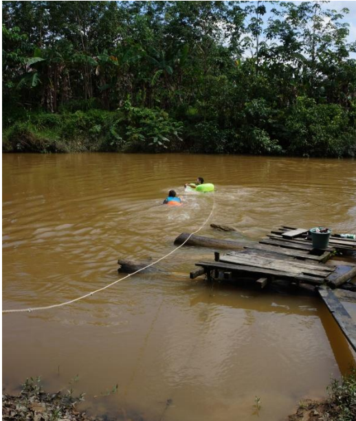
Figure 4.3.1.1 - Swimming over the river at station 2 to tie the one-meter knotted rope to the other river bank.
