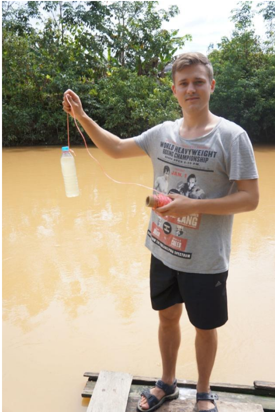
Figure 4.3.3.1. - Float tied to short bamboo handle, used as velocity measurement at station 1 and 2.
