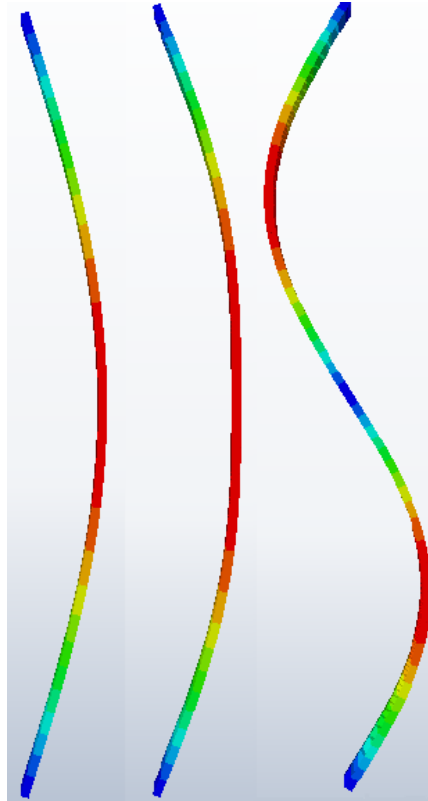
Figure 5.11 From left to right the stiffness of the brace is 0 to 29200 N/m. For case A.
