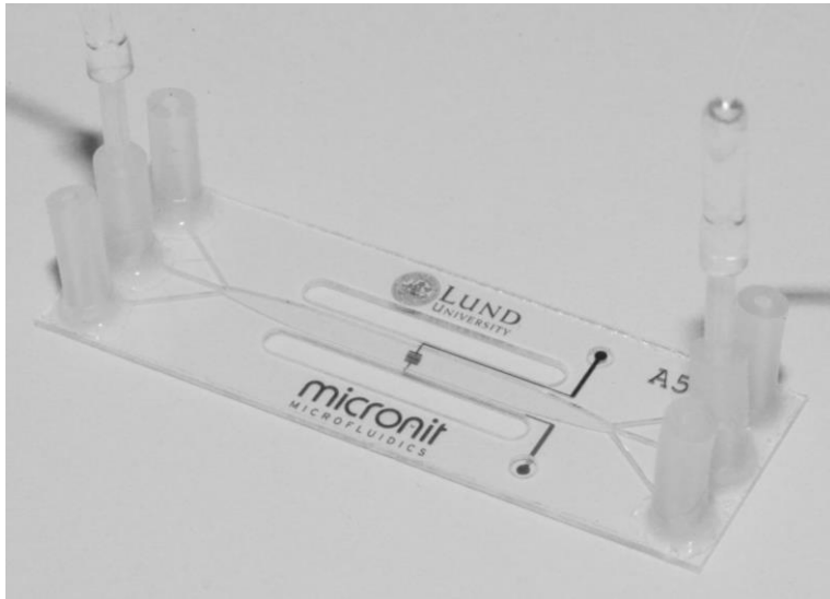
Figure 5.4. Image of the glass chip. The two circular metal areas to the right of the middle are the connection sites to the electrodes (electrode pads). One can be contacted from the top side of the chip and the other from the opposite side. In the middle of the channel the electrodes can be seen. At the right and left sides of the chip the three inlet and three outlet tubing are glued to the chip.
