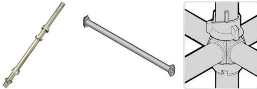
Figure 3.2 – CUPLOK components and the CUPLOK connection system (BRITEK Ltd)
