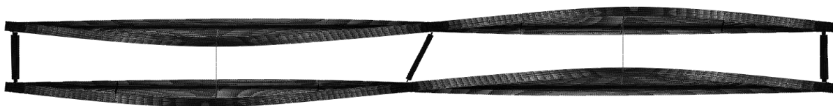
Figure 7.4 – First mode shape of beam system with bracing just at supports
