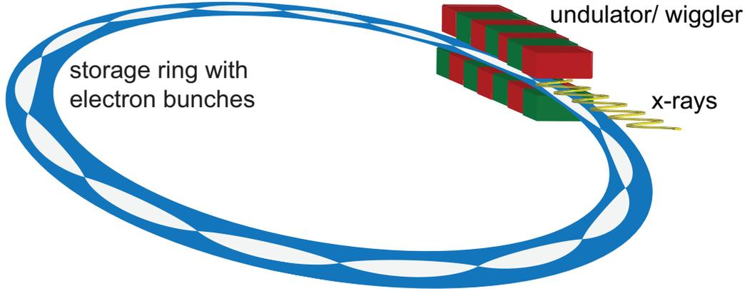
Figure 2.1: Simplified schematic of a synchrotron radiation source. Relativistic electrons circulate in the storage ring. By passing through the alternating magnetic field of the insertion device, here an undulator or wiggler, electrons are forced onto an oscillating path, which leads to the emission of synchrotron radiation.
