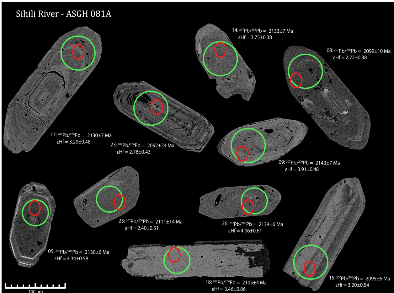
Fig. 16. BSE of detrital zircon from Sihili river (ASGH 081A). Red ellipsoids mark the spot for U-Th-Pb analyses and green circles the spot location for Lu-Hf analyses.
