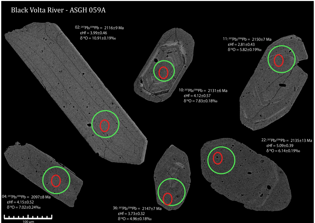
Fig. 14. BSE of detrital zircon from Black Volta river (ASGH 059A). Red ellipsoids mark the spot for U-Th-Pb analyses and green circles the spot location for Lu-Hf analyses.
