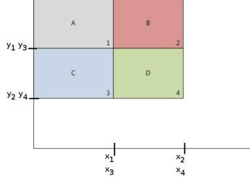
Figure 4: The sum in area A is I(x_1, y_1) . To calculate the sum in area D, its equal to I(x_4, y_4) + I(x_1, y_1) - I(x_2, y_2) - I(x_3, y_3)
