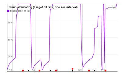
**Figure 7.14:** Target bit rate by TCP-Illinois during the 3 min alternating test. The interval the algorithm is running has been doubled to one second. We can see that Illinois is acting more stable than the previous graph.
