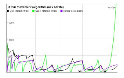
**Figure 7.1:** Target bit rate during the 3 min movement test at AXIS, We get a lot of packet loss here but we can see that the algorithms follow the expected behavior after wards
