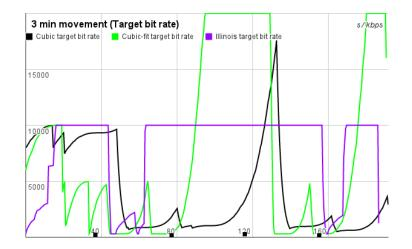
**Figure 7.12:** Target bitrate after introduction of PLL. The algorithms run smoother than without the PLL.
