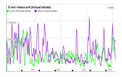
**Figure 7.9:** Here we can see that the actual bitrate is allowed to be lower than the target bitrate if the rate controller sees that there are little motion.
