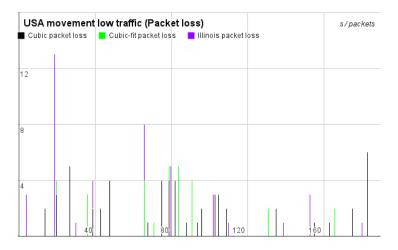
**Figure 7.33:** Packet loss during the movement test to USA. We can see that we got a lot less packet loss during low peak hours.
