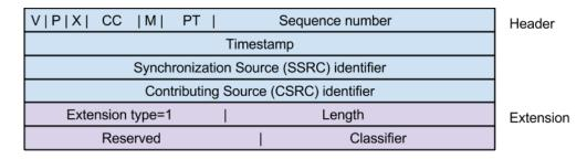
**Figure 2.2:** The structure of an RTP packet. Every bar is 32bit long. V stands for Version, P padding, X Extension, CC CSRC count, M marker and PT for payload type
