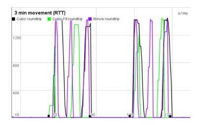
**Figure 7.7:** The round trip time increases a lot when we limit the switch wost likely strengthening our assumption that hybrid algorithms should perform better.
