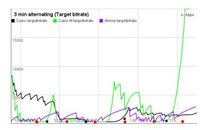
**Figure 7.2:** Target bit rate during the 3 min alternating test at AXIS.
