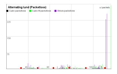
**Figure 7.16:** Packet loss during alternating movement in Lund. We can see that packet loss occur in conjunction with movement. The peaks of packet loss in the end of the graph is from when we shut down the stream during the tests(it expects that it should receive a lot of packages but since we interrupt the stream they never arrive).
