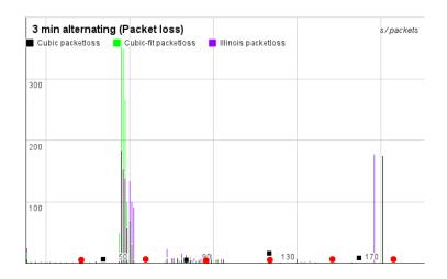
**Figure 7.4:** Alternating movement packet loss. Note that the we receive no packet loss when movement starts but after a few seconds with movement and limiting of the switch we got a lot of lost packets.
