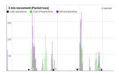
**Figure 7.3:** Movement packet loss. It is easy to see that the most of the packet loss occur directly after we limit the switch.
