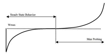
Figure 6.1: TCP-CUBIC growth curve after packet loss
