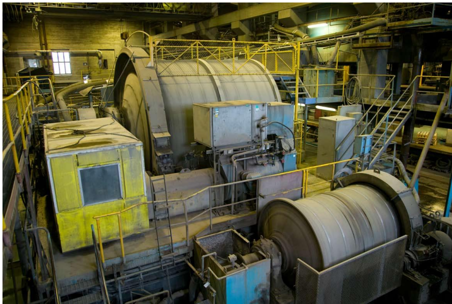
Figure 2-1: Mills in the extraction plant at Garpenberg (H. Aitahmed-Ali (Boliden), personal communication, 2013-10-31).
