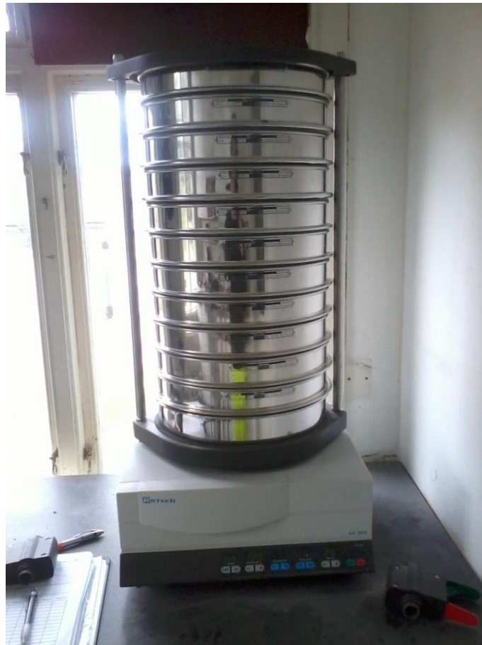
Figure 5-22: Sieving apparatus and meshes, 2013-09.
