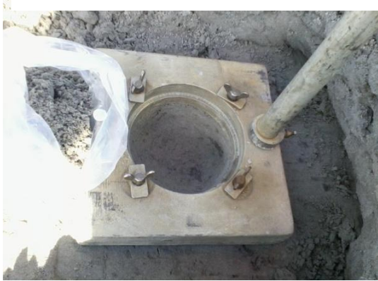
Figure 5-18: Hole dug under the balloon densitometer.
