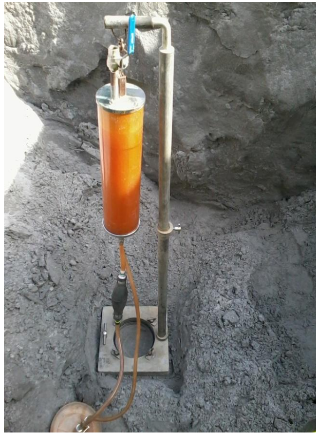
Figure 5-17: Volume of hole under the balloon densitometer was determined.
