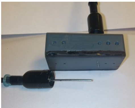
Figure 2.5: Fibre holder with the two optical fibres
