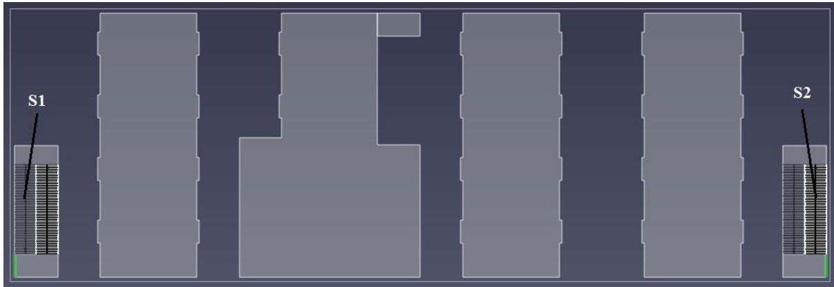
Figure 4.3. Representation of the lobby core with stair 1 and 2 as available egress components. The core includes the different elevator banks for the different zones of the building, which are only used for regular circulation (not during evacuation).
