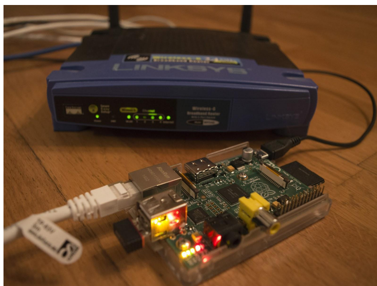
Figure 4.1: A Raspberry Pi Revision B running the IBM software TPM with remote access over TCP/IP.
