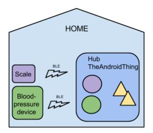
**Figure 2.2:** Simplified architecture of the setup of the hub in the kidney project. Each BLE peripheral is connecting to PalCom through a intepreter service (circles), which in turn is used by assemblies (triangles) to send data to a monitoring centeral.
