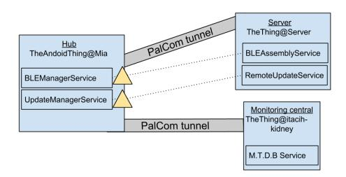
**Figure 3.6:** The setup prepared for automatic installation and update of BLE services. The two triangles indicate assemblies connecting the services on the hub to their corresponding service on the server.
