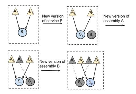
**Figure 3.1:** Switching to version two of service S when all assemblies (A and B) have been updated and assemblies and services in version one are stopped (dark grey).
