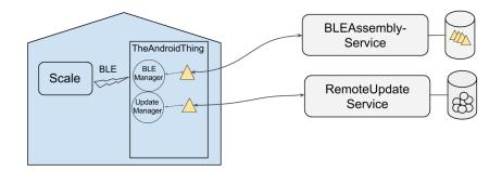
**Figure 3.4:** An overview of the main components of the implementation. Where assemblies (triangles) and services (circles) are distributed on demand.
