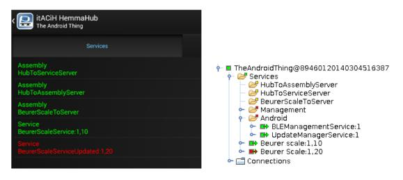
**Figure 3.10:** A new version of BeurerScaleService is loaded and currently in a non-operational state, because no assembly is connected. The prevous version is still fully operational and thus connected to the scale. To the right we see the same hub from the PalCom browser.
