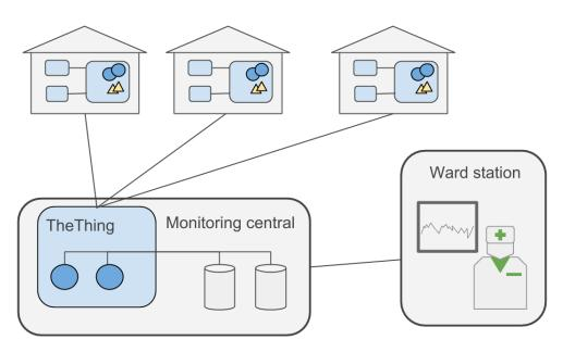
**Figure 2.1:** The hubs running at the patients' home are connected through PalCom tunnels to a TheThing on a monitoring central. Each hub can then send measurements to a receiver service on the monitoring central for storage (cylinders), these serivces (circles) are connected though assemblies (triangles). An itACiH application retrives and presents the measurements for medical personnel.
