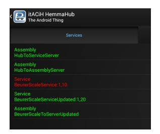
**Figure 3.11:** The update of the Beurer scale service is now completed. Version 1.10 is in a non-operational state (red) while version 1.20 is fully operational (green) and has taken over the communication with the scale.
