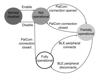
Figure 3.5: The different operating states of a BLE service.
