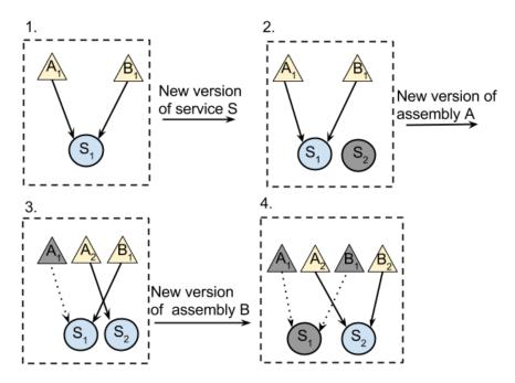
**Figure 3.2:** Switching to new versions when two versions are executing simultaneously. Notice in step three, where  $A_2$  uses the new version of S while  $B_1$  still use the old version. Having two versions running simultaneously is not always meaningful for some bound services such as BLE services, where only one of the two versions can be connected to the BLE peripheral.
