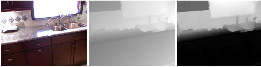
Figure 2.6: An RGB-D image with the RGB content to the left, D content in the middle and to the right the data term corresponding to the RANSAC proposal with the most inliers.
