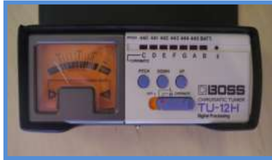
Picture 1: Analogue chromatic tuner I used for the acoustic analysis
