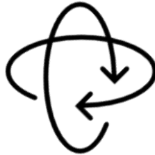
Figure 2.4: Illustration of pan (horizontal) and tilt (vertical) movement.
