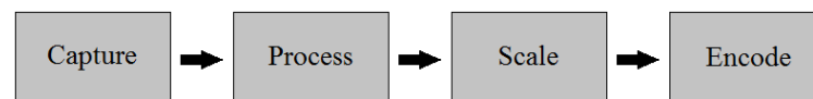
Figure 8.3: The four steps of generating an image. Overlays are added in the third step, Scale, before the image is encoded.
