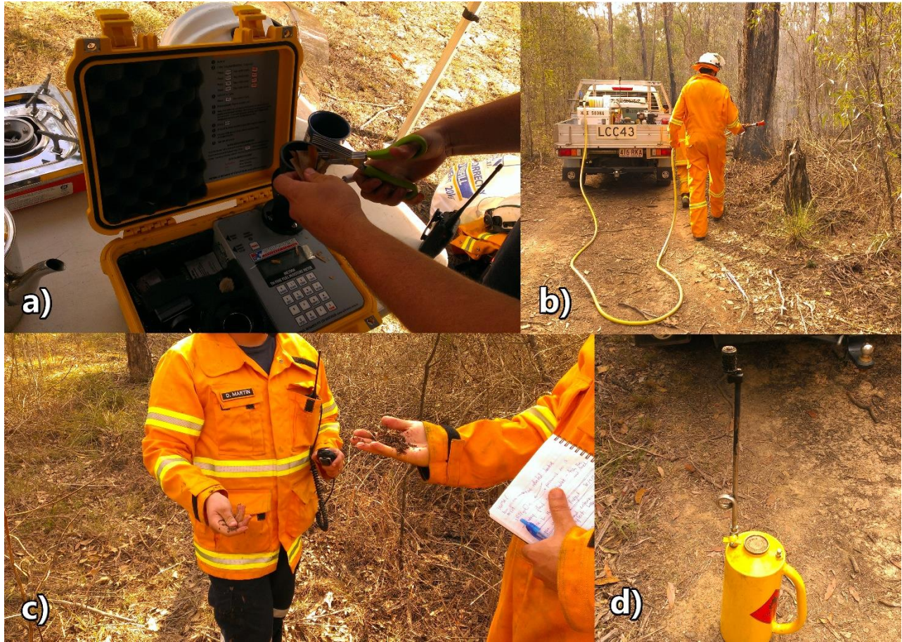
Figure 3-4- a) moisture meter; b) extinguishing process by means of a pump car and water hose; c) eye examination of the fuel moisture; d) driptorch
