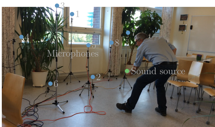
Figure 4.1: Experimental setup with one moving sound source and eight microphones.
