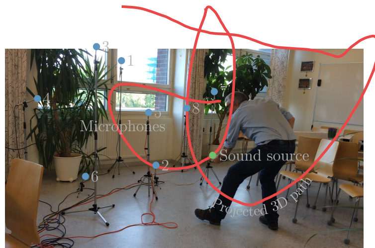
Figure 5.3: The 3D path from Figure 5.2 projected at video recording of the experiment. The video is presented in Appendix B.
