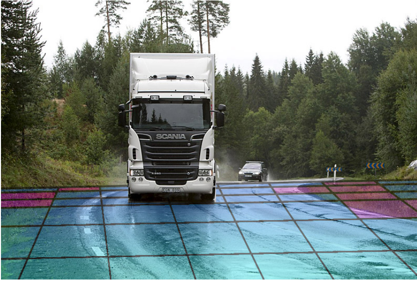
Figure 3.6 An elevation map illustrated. The color shows the elevation of the square: blue indicates a higher elevation and red indicates a lower elevation. © Scania CV AB
