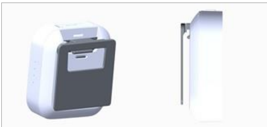
Figure 4.14 Narrative snap-fit case
