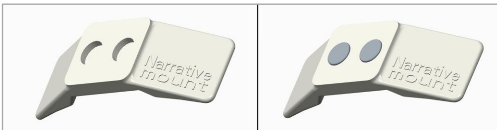
Figure 5.13 Two magnets on the flat surface of the bottom plate, where the ball-joint and the camera case will be attached
