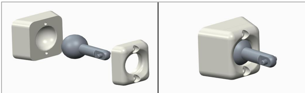
Figure 5.15 How the ball is placed in the ball-joint
