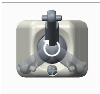
Figure 5.18 The rotation possible with a ball-joint
