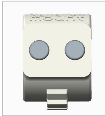
Figure 5.5 Two magnets on the flat surface of the bottom plate, where the ball-joint and the camera case will be attached
