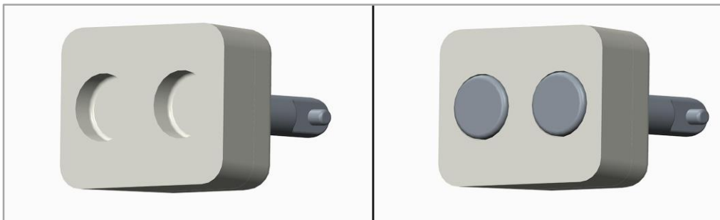
Figure 5.17 Magnets on the underside of the ball-joint
