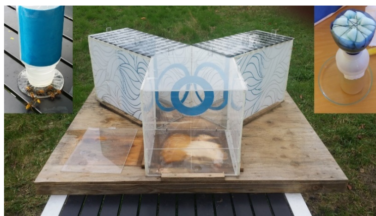
Figure 2. The experimental apparatus, consisting of a Y-maze screwed to a wooden sheet. The two insets represent the two types of feeders used: left – feeder used during training, right – feeder used during the experiments.
