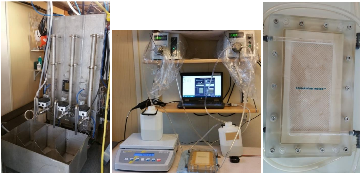
Figure 3.4. Alfa Laval MF membranes (left), biomimetic membrane FO filtration set-up (center) and the Aquaporin membrane itself (right) Photos by: Hey, 2015.
