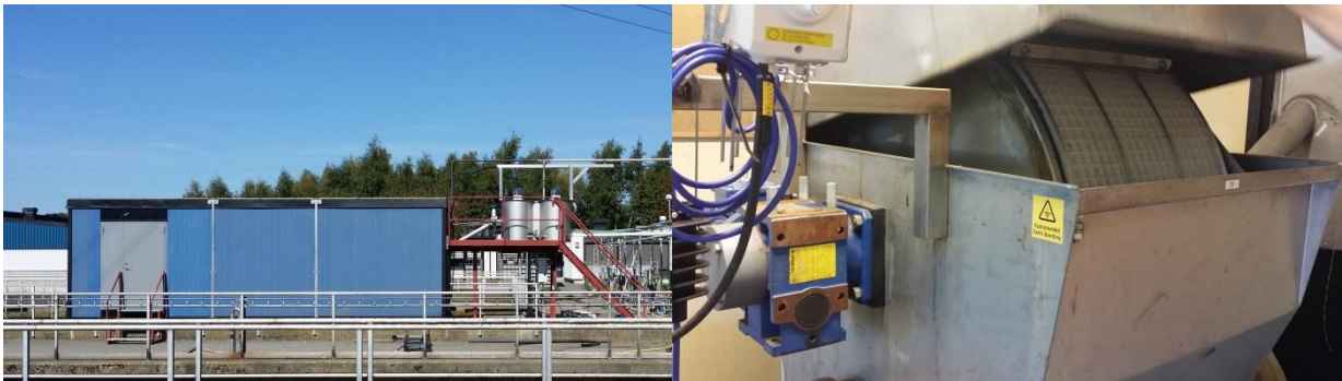
Figure 3.3. Photo of the pilot plant taken from the outside (left) and of the Hydrotech drum filter (right). Photos by: Hey, 2014.
