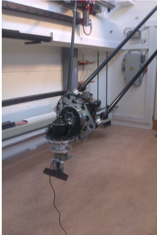
Figure 6.2 L2 Gantry Tao Robot with mounted Xtion Asus Pro Live RGB-D camera.
