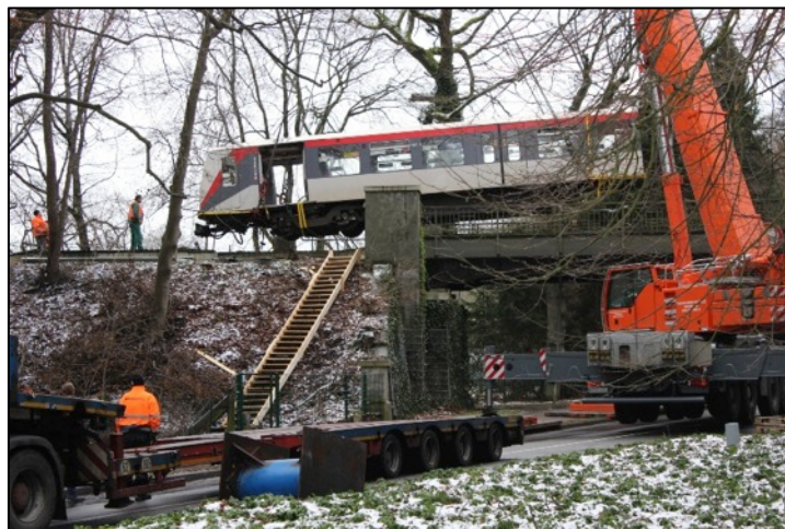
Fig. 4: Hochbahn metro coach derailed by a fallen tree in Großhansdorf close to Hamburg. Photo: © Monika Veeh / ahrensburg24.de
