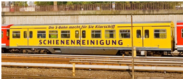
Fig. 8: Fed by past weather experience, Hamburg's operators have developed response strategies. The picture shows a maintenance coach removing leaves from the S-Bahn rails. Wet leaves impede braking effectivity in autumn.
